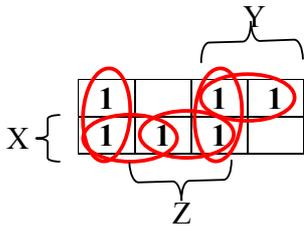
$$f(x,y,z) = y'z + xy' + xz + yz + x'y + x'z'$$
